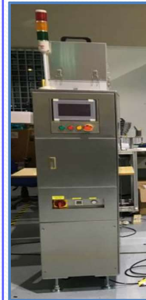
SLOT Magazines loader, buffer, unloader
