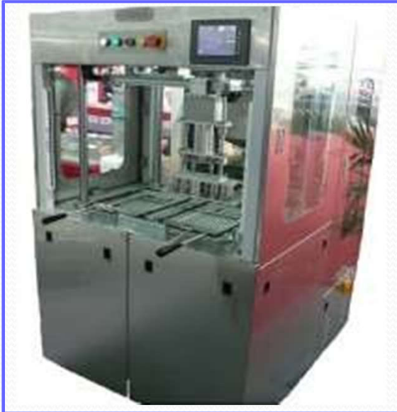
Auto Pellet Loader for IC MGP Molding
