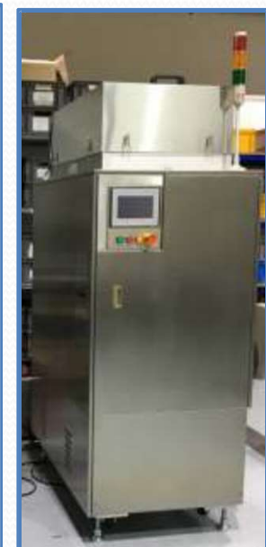
SLOT Magazines loader, buffer, unloader
