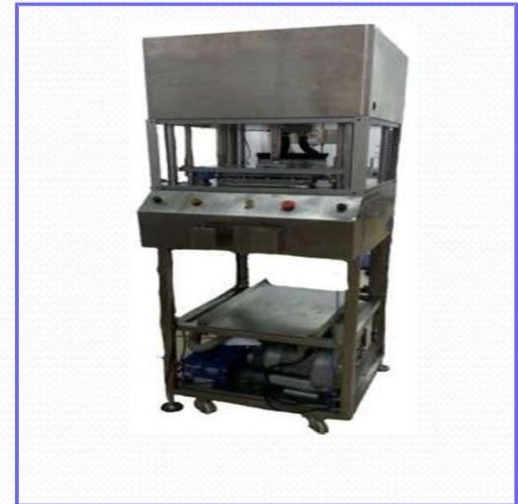
Semi Auto Deculler for IC MGP Molding
